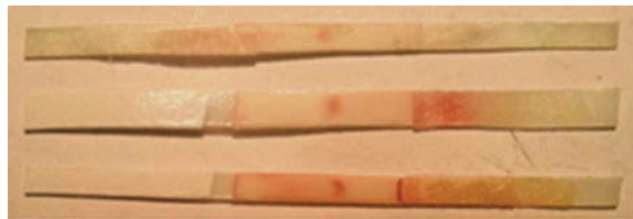
Figure 4. Gold conjugation of three monoclonal antibodies. Five monoclonal Ab conjugated with nanogold as detection Ab and as capture Ab concentration of troponin I is 1 ng/mL.
