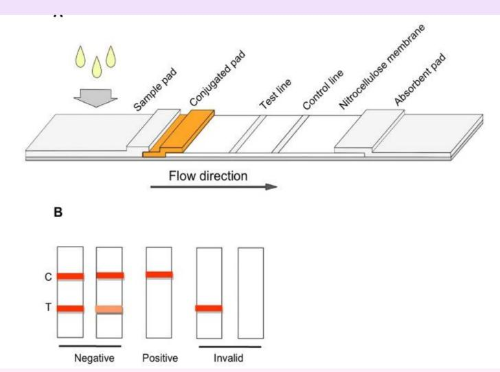
Schematic diagram of the immunochromatographic test strip. •Notes: (A) The preparation and assembly of the immunoassay test strip. (B) Result judgment of the test strip. C, control line; T, test line.
